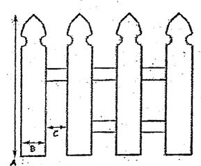
$A = 42^{\circ}$  (with an installed length of as more than 48).  $B = 3.3/8^{\circ}$   $C = 2.1/2^{\circ}$
